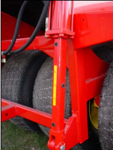
Figure 6: Hydraulic cylinder support in place
