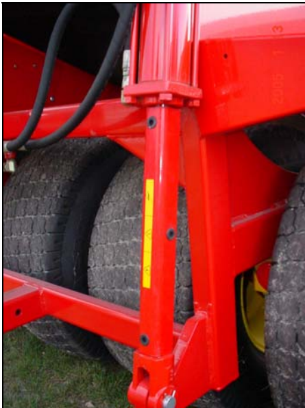
Figure 30: Hydraulic cylinder support in place
