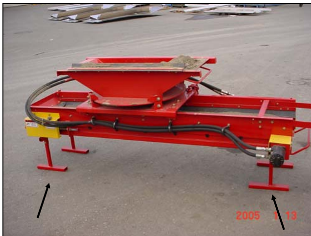
Figure 27: Cross conveyor on storage stands
