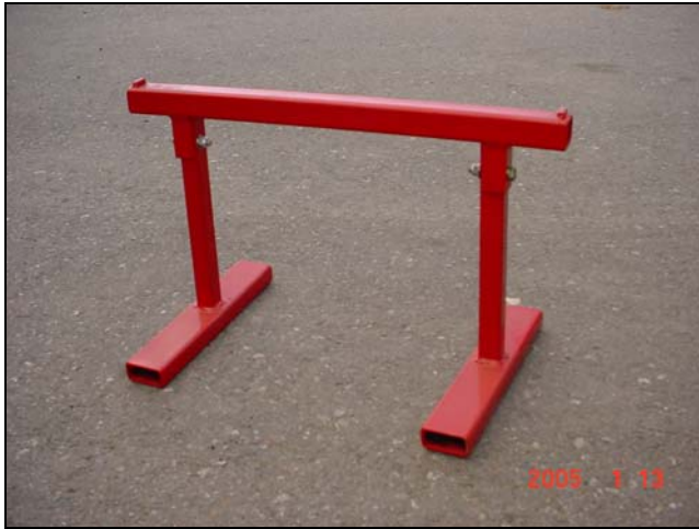
Figure 29: Cross conveyor storage stands
