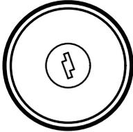
The key switch controls the engine and electrical system. A key is used to select the key switch position. The key can only be inserted or removed when the key switch is set to OFF. Vehicles with this key switch are pedal-start vehicles.
