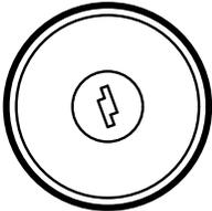
The key switch controls the engine and electrical system. A key is used to select the key switch position. The key can only be inserted or removed when the key switch is set to OFF. Vehicles with this key switch are key-start vehicles.
